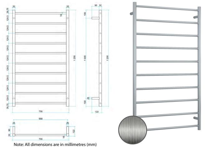
This rail has Multiflex wiring which means that there is a connection point on both the left and right hand side of the rail and the lead can be connected to either side. Being a dry element rail, this can be mounted either way up meaning the wiring can be from any of the four mounting points.
