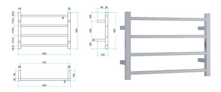
This rail has Multiflex wiring which means that there is a connection point on both the left and right hand side of the rail and the lead can be connected to either side. Being a dry electric element rail, this can be mounted either way up meaning the wiring can be from any of the four mounting points.
